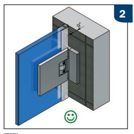
To prevent tilting of the rotational axis, always mount the shower door hinge in such a way, that its entire surface contacts the tile. \*When using sealing profil 8861KU-8
