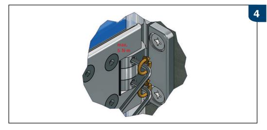
Once the door wing is aligned and all sealing profiles are fitted, the zero position can be a justed. Tighten the set screws alternately to the specified torque; retighten after approx. 15 minutes. Those grub screws can additionally be fixed with thread locker. The angled allen key SW2,5 No. 8129ST8 has been included. WARNING: This key should be used for 2 assemblies only!
