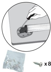
Screw the bracket to the table top, using all the enclosed screws.
